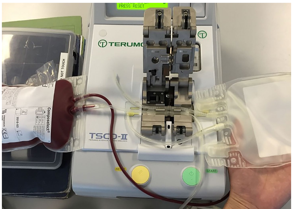
Figure 5. PRBC unit split being into another smaller unit using the tube welder.
