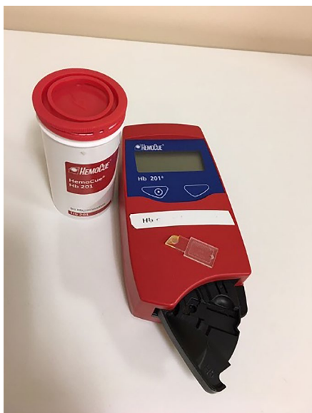
▲ Figure 2. Hemocue® – haemoglobin point-of-care machine used to check the blood donors haemoglobin levels prior to donation.
