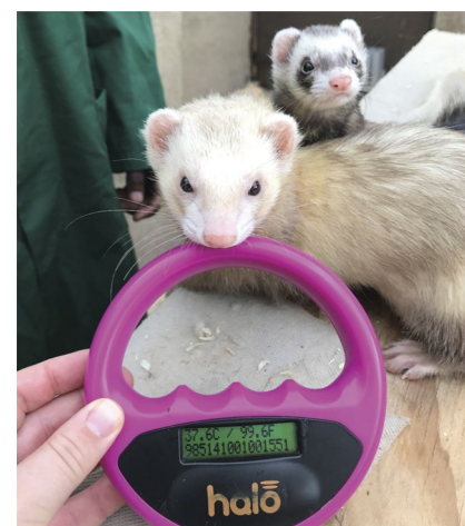
Figure 3. A Halo microchip scanner used to record ferret microchip temperature in a willing volunteer.
