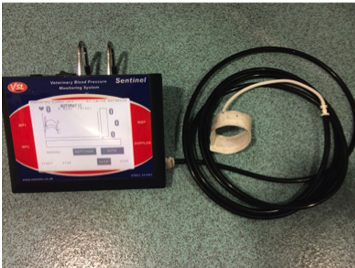
Figure 2. An oscillometric device for measuring blood pressure
