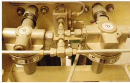
Figure 10: Diagram of flow control valve and flowmeter (image courtesy of Al-Shaikh & Stacey)
