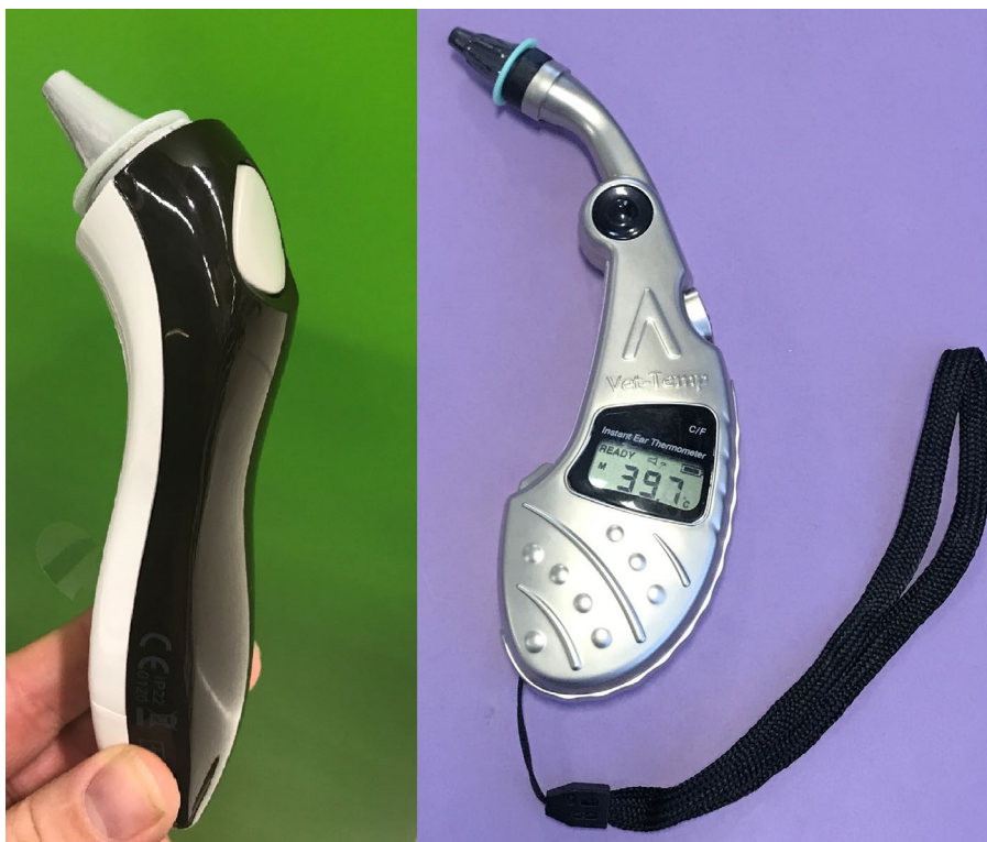
Figure 3. A human aural thermometer alongside a VetTemp® aural thermometer with probe cover in place
