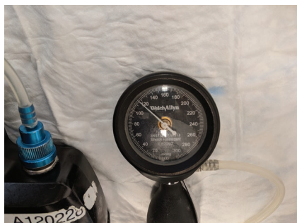
Figure 4. A leak tester is attached and pressurised to the correct level to check for leaking.
