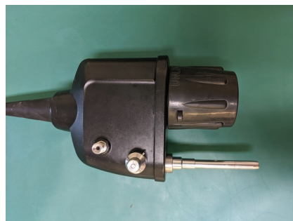
Figure 2. A waterproof cap is placed on the end of the umbilical cord prior to cleaning.
