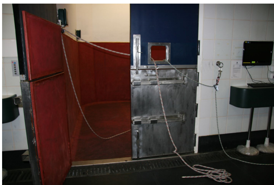
Figure 3. Recovery room with rope-assisted recovery system: the red rope connects to and supports the head while the green rope with friction-brake climbing device (PetzlGrigri) supports the tail; note the padded walls and floor
