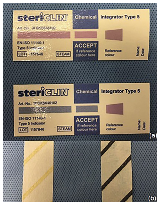
Figure 4. The figure showing indicator strips (a), changing from blue to pink; and autoclave tape (b), changing from yellow to brown to indicate that adequate temperature, time and pressure have been achieved.
