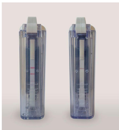
▲ Figure 2. PCRRun™ detection device used to detect a qualitative PCR result
