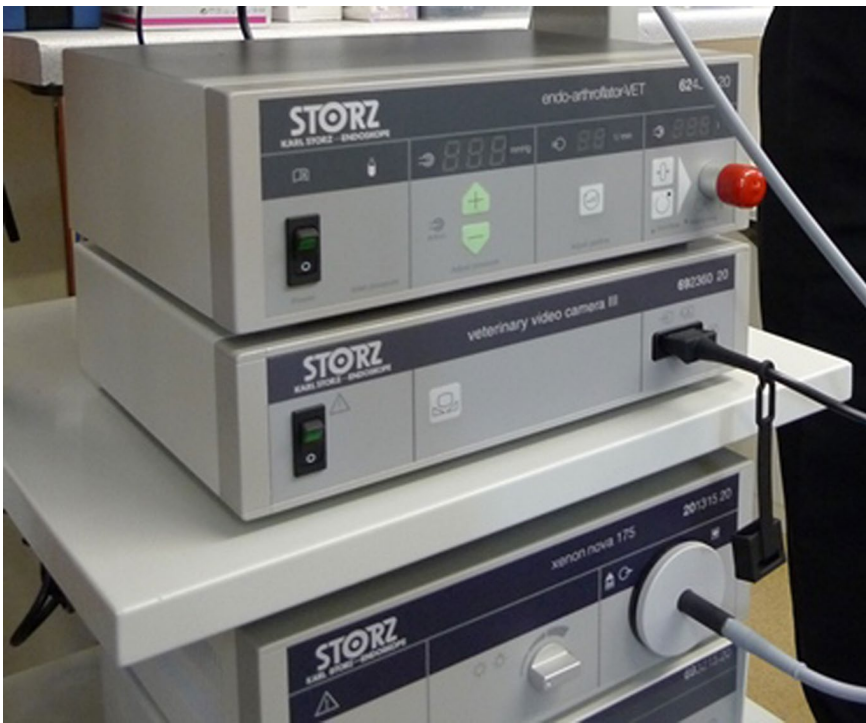
▲ Figure 2: Laparoscopy tower – top to bottom: CO 2 insufflator, camera, light source
