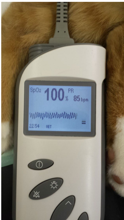
▲ Figure 6a. A SpO 2 reading from a poorly placed pulse oximeter probe. Note the poor plethysmographic pulse waveform. This type of waveform should signal to the anaesthetist that the SpO 2 reading is unlikely to be accurate and that the probe placement should be checked
