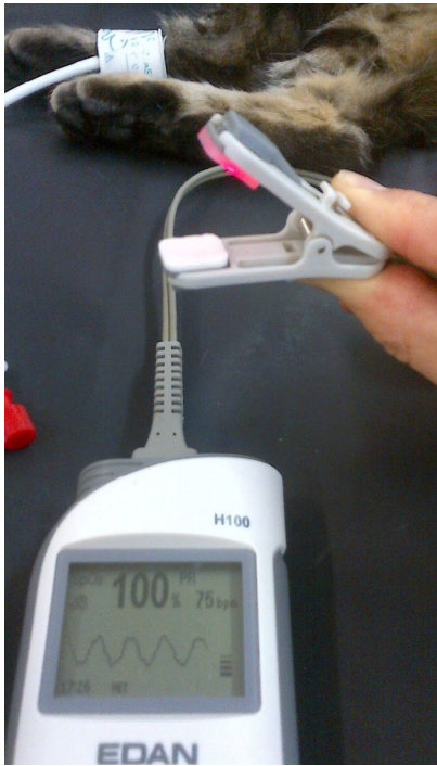
▲ Figure 5. A convincing pulse waveform and SpO 2 reading given by ambient lighting. The pulsatile nature of fluorescent lighting can cause erroneous readings. Many modern probes are able to subtract this effect, but budget models may be effected. Covering the probe to block out ambient lighting can help eliminate this error
