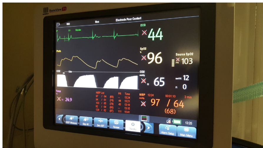
▲ Figure 7. Double-counting of the pulse rate caused by a large “rebound pulse” secondary to elastic recoil of the major vessels (note the disparity between the false pulse rate in yellow from the pulse oximeter and the correct heart rate from the ECG). A high rebound pulse is common following medetomidine administration and can be misread by the monitor. The plethysmographic pulse trace should be checked and cross-referenced with other monitoring (e.g. manual pulse count or ECG) before the numbers are believed and recorded
