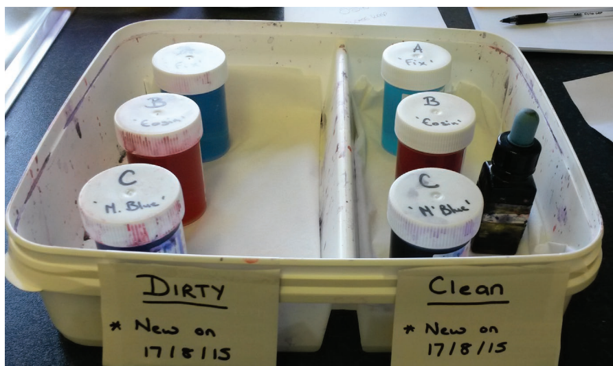
▲ Figure 5: Separate staining sets for 'clean' and 'dirty' slides helps to minimise stain contamination thus improving the accuracy of microscopic analysis
