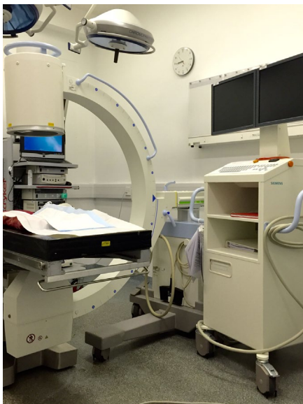
▲ Figure 4. C-Arm fluoroscopy unit set up in theatre, showing the X-ray tube and image intensifier positioned above and below the operating table
