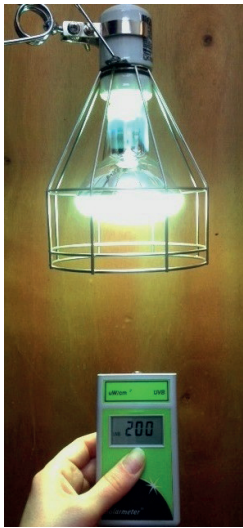
Figure 7. A UVB solarmeter used to test UV lamps
