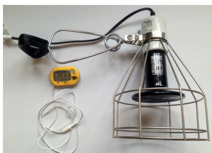
▲ Figure 5. A ceramic lamp used to provide heat at night time, and a digital thermometer probe
