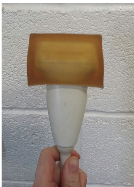
Figure 2. A linear-array transducer with stand-off pad
