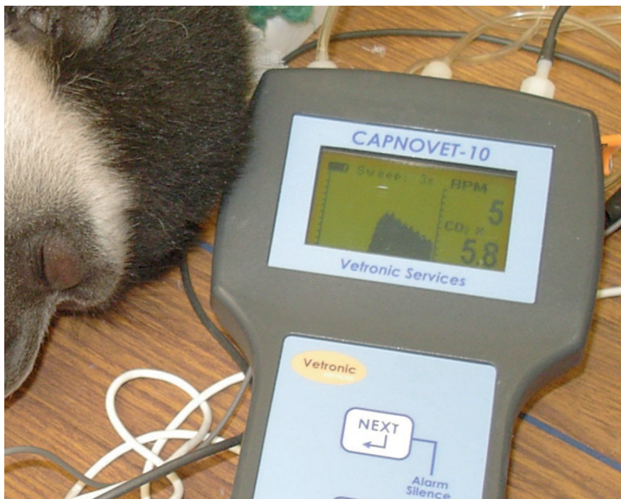
Figure 5. The waveform starts to fall off as the sidestream unit brings in diluting fresh gas
