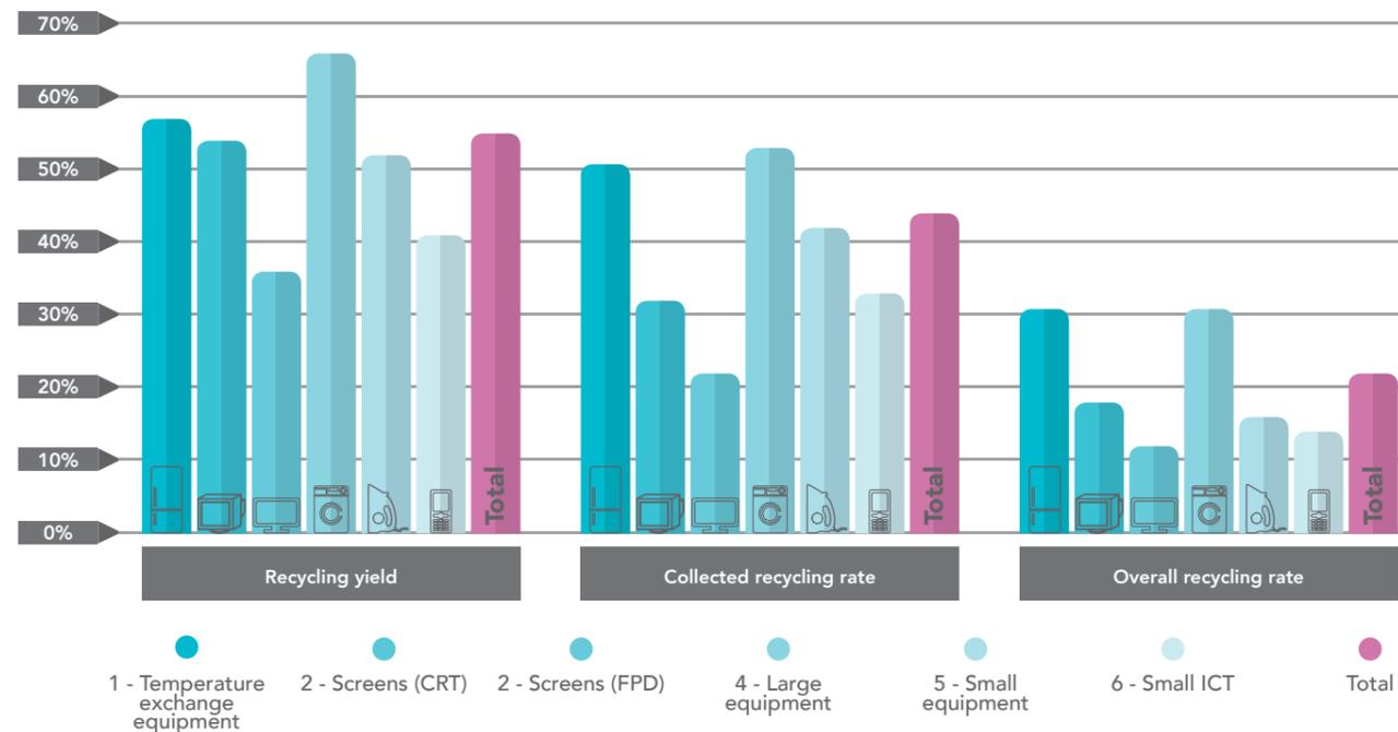
The **recycling yield** ranges between 36% (FPD screens) and 57% (TEE), with a yield of 55% across all WEEE categories. This means that, **on average, 55% of WEEE plastics entering WEEE plastic recycling facilities will actually be turned into regranulates.**
