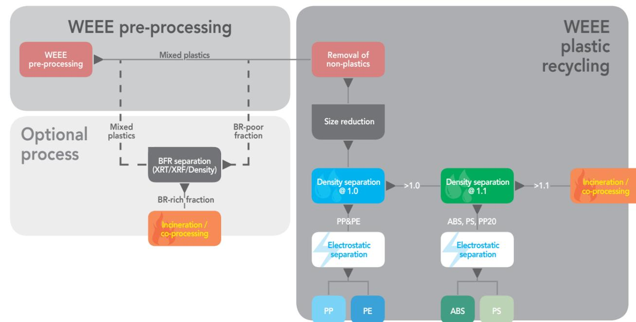
Figure 12 : Conventional WEEE plastic treatment processes
